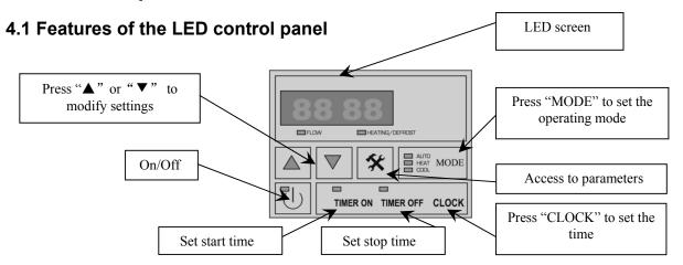
With the "On/Off" key "\_\_\_", the heat pump is turned on or turned off (stand-by status). If the LED next to this key lights up, the heat pump is turned ON.
