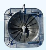
Solar Pod operates by harnessing the free energy from the sun and transferring it into your pool water, its "heat trap" technology with glass house effect captures energy within the ultra-clear polycarbonate dome and transfers heat to its polycarbonate heat exchanger. Solar Pod's clear dome also reduces heat loss from its heat exchanger caused by wind exposure.
